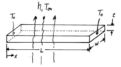
For W=1 m, t=0.01 m, L=3 m, and given the copper properties c=393 J/kgK, k=386 W/mK,  $\rho=9000$  kg/m<sup>3</sup>, and knowing that  $T_0=300^{\circ}$ C and  $T_{\infty}=20^{\circ}$ C, and that the conductive heat transfer between the fin and the objects cooled corresponds to:
