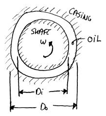
The shaft rotates at a speed  $\omega$  (in rad/s), and the oil has a density  $\rho$  (in kg/m<sup>3</sup>), a viscosity  $\mu$  (in kg/ms), and a thermal conductivity k in (W/mK). Knowing that there is heat generation *inside the shaft* of S (in W/m<sup>3</sup>) and that the temperature of the casing is of  $T_o$  (in °C), do the following:
