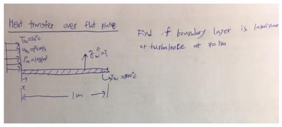
The example wanted whether flow is turbulence or laminar at x=1m. While you give this example, you missed the assumptions and let assumptions as blank. So, i try to fill it out and here's my idea. : 1. Steady-state flow 2. Plate should be flat and thin plate  $3.\rho\rho$ , c, k are constant 4. EcEc<<1Pr I wonder whether my guess is right or wrong.
