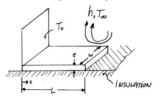
Knowing that the fin tip is **not** insulated, that  $W \gg L$ , and that there is no heat transfer between the fin and the table, do the following:
