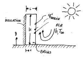
For H=1 m, L=0.1 m,  $T_{\infty}=27^{\circ}$  C,  $P_{\infty}=1$  atm, and an incoming radiation heat flux from the sun equal to  $q''_{\rm radin}=700~{\rm W/m^2}$ , and an emissivity factor of the bricks of  $\epsilon=0.5$ , do the following:
