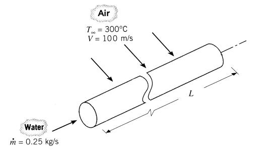
Over its entire length of L=6 m, the pipe is heated on its outside surface by a cross flow of air at a pressure of 1 atm, a temperature of  $300^{\circ}$  C, and a speed of 100 m/s. For a pipe of negligible wall thickness (resulting in essentially equal internal and external pipe diameters), calculate the bulk water temperature at the pipe exit.
