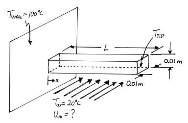
There is a cross-flow of a fluid over the bar as shown in the figure above:  $T_{\infty}=20^{\circ}\,\mathrm{C}$ , and  $U_{\infty}$  is unknown. The fluid properties may be assumed constant at the following values:
