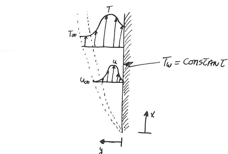
For a gas, neglecting all shear stresses except the one normal to the wall but including the body force due to gravity the x-momentum equation becomes:
