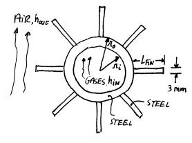
Each fin is 3 mm thick with a width of 1 m (spanning the length of the cylinder). You wish to minimize the length of the fins  $L_{\rm fin}$  as much as possible to keep the weight of the combustor down while resulting in sufficient cooling so that the combustor temperature anywhere (i.e., anywhere within the steel) doesn't exceed 800 °C. What would be the optimal fin length that would accomplish this? Specifically, given the following air, gases, and steel properties:
