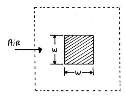
The air in the freestream has a Mach number of 2.5, a pressure of 5 kPa, and a temperature of 300 K. The width of the cross section is of W = 0.1 m. The goal is to determine the drag coefficient  $C_D$  as accurately as possible while using as few computational resources as possible. Design a mesh that is optimal for this problem (i.e., that will yield the smallest product of error and computational time). Set the viscosity and thermal conductivity to zero.
