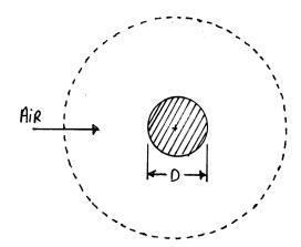
The air in the freestream has a Mach number of 2.5, a pressure of 5 kPa, and a temperature of 300 K. The diameter of the cylinder is of D=0.1 m. The goal is to determine the drag coefficient  $C_D$  as accurately as possible while using as few computational resources as possible. Design a mesh that is optimal for this problem (i.e., that will yield the smallest product of error and computational time). Set the viscosity and thermal conductivity to zero.
