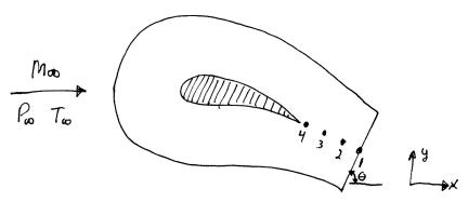
The freestream properties correspond to  $M_{\infty}=0.7, T_{\infty}=300 \text{ K}, P_{\infty}=1 \text{ atm},$   $\theta=70^{\circ}$  and the properties on the nodes at the iteration n are as follows:
