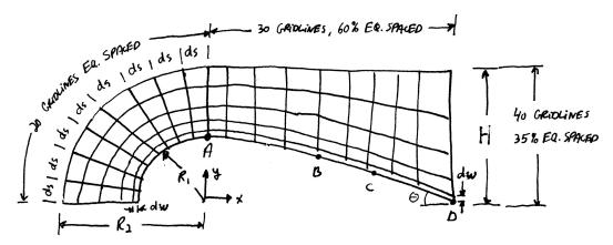
given the dimensions  $dw=10^{-4}\,$  m,  $R_1=0.5\,$  m,  $R_2=1\,$  m,  $x_{\rm A}=0, y_{\rm A}=R_1$ ,  $x_{\rm B}=0.5\,$  m,  $y_{\rm B}=0.9R_1, x_{\rm C}=1\,$  m,  $y_{\rm C}=0.7R_1, x_{\rm D}=2\,$  m,  $y_{\rm D}=0, H=R_2$ , and  $\theta=20^\circ$ . Notes:
