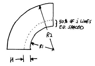
with  $R_1 = 1$  m,  $R_2 = 2$  m and H = 0.1 m. Make sure that the grid is uniformly-spaced along i.
