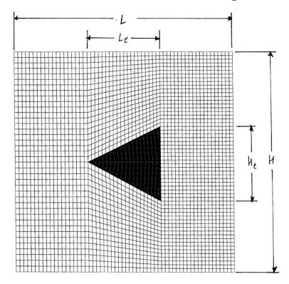
The flow infinitely far from the triangle has a temperature of 300 K, a pressure of 20 kPa, and a velocity (in the right direction) of 600 m/s. Knowing that the grid is made of 60 gridlines in each dimension, and that L=2.1 m, H=2.1 m,  $L_{\rm t}=0.7$  m,  $H_{\rm t}=0.7$  m, that the grid on each side of the domain is uniformly spaced, and that the triangle is centered within the domain, write the code needed within the Grid() module to simulate this problem.
