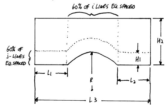
The mesh should have 70 grid lines along i and 70 grid lines along j with  $L_1=0.3$  m,  $L_2=0.3$  m,  $L_3=1.0$  m, R=0.7 m,  $H_1=0.1$  m, and  $H_2=0.5$  m.
